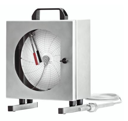
Chart Recorders are the industry standard for accurate, reliable measurement and recording of pressure and temperature or a combination of those (max. 3-pens) in a wide variety of applications.
