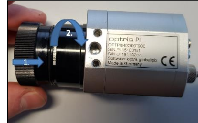
Figure 13: Inserting the lens
