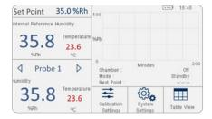
A 4.3" LCD touchscreen runs a powerful UI, which displays all measured values from the reference and probes under test, along with a graphical trend indication of chamber stability. It is also capable of automating complete validation procedures with ease and providing a complete logged output in csv format straight to your USB memory device, to minimize the time you spend taking readings.
