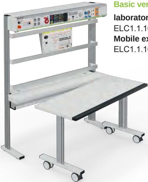
Example 2: Laboratory bench: ELC1.1.1641.C 1600 x 400 x 780 mm. Table type 1.1. ergo-line worktop (laser edge). Mobile extension table: ELC1.1.1663A.T 1600 x 600 x 780 mm. Worktop alu-line (laser edge). Structure: Extended L-profiles. 19-inch cockpit, equipped with the basic and elneos six device series. 2-row experiment frame between the base profiles. Cable aperture sockets embedded in the table top, open cable tray underneath the table.
