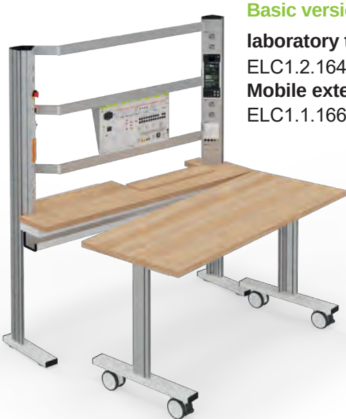
Example 3: Laboratory bench: ELC1.2.1648.C 1600 x 400 x 780 mm. Table type 1.2 with 180° cable flap. Optional split cable flap. Multiplex worktop. Mobile extension table: ELC1.1.1668A.T 1600 x 600 x 780 mm. Worktop multiplex. Connectors each in graphite black, RAL 9011. Structure: Extended L-profiles with Expand 2 profiles on the left and right, fitted with the acto and elneos six compact device series. 2-row experiment frame between the base profiles.
