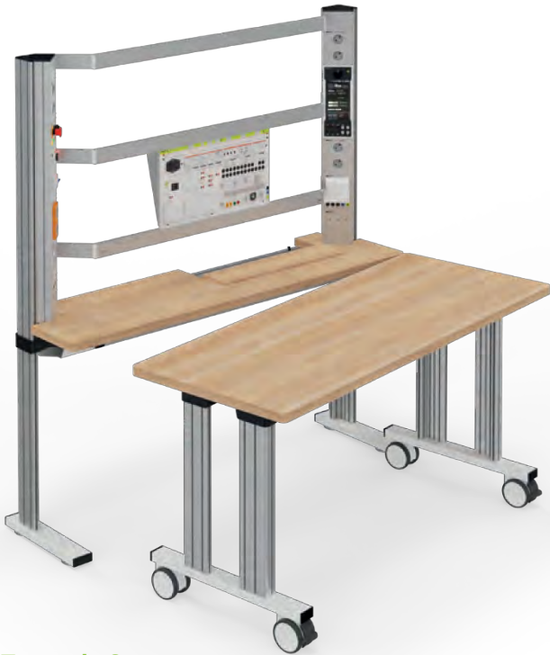
Example 3: Laboratory bench: ELC1.2.1648.C 1600 x 400 x 780 mm. Table type 1.2 with 180° cable flap. Optional split cable flap. Multiplex worktop. Mobile extension table: ELC1.1.1668A.T 1600 x 600 x 780 mm. Worktop multiplex. Connectors each in graphite black, RAL 9011. Structure: Extended L-profiles with Expand 2 profiles on the left and right, fitted with the acto and elneos six compact device series. 2-row experiment frame between the base profiles.
