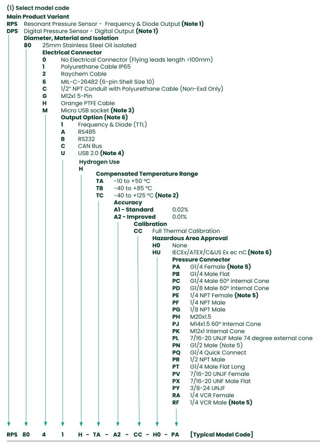
**Note 1:** RPS variants require Output Option Code '1'. DPS variants require Output Option Code 'A', 'B', 'C' or 'U'. **Note 2:** Requires Output Option Code '1' or 'C' and Electrical Connector Codes '0', '2', '6', 'G', or 'H'.
