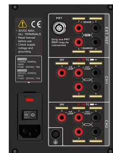
Quick-Push connectors for reference and UUT channels easily accept banana, large and small spade lugs and bare wire connections
