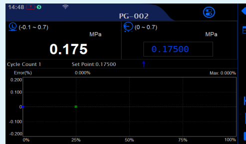
Pressure gauge / transmitter / switch calibration
